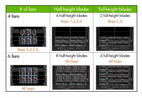
Figure 5. The c3000 Enclosure fan bay and device bay population guidelines
